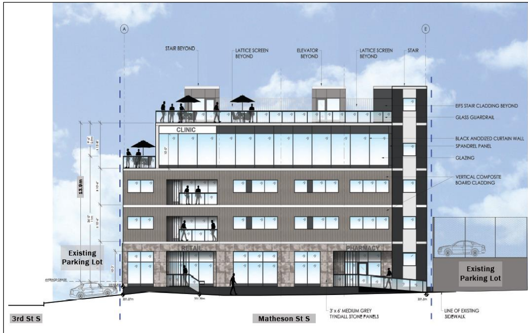
Figure 7: East Elevation - View from Matheson Street South
